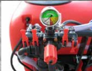
Pressure Regulator Valve with Manual Controls
