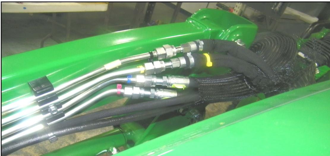
7. At the front of the loader, open the clamp on the Front Manifold open, pass it around the loader cross tube. Position the Manifold on top of the flat cover of the cross tube. Insert the tail of the mounting clamp into the screw housing. Take up excess length, but leave it loose.
