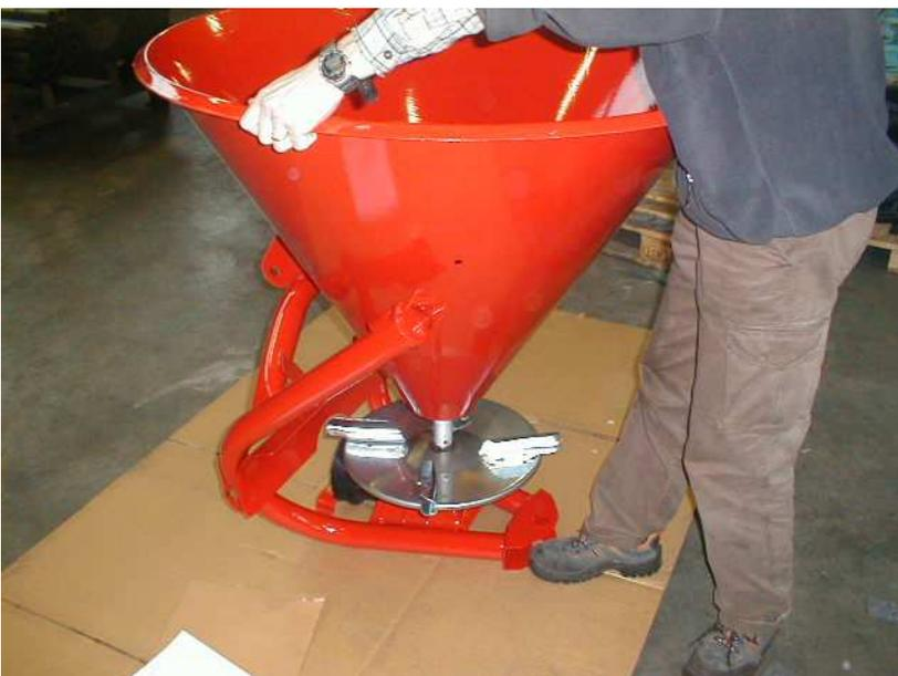
5) put the hopper in by centring the hole
