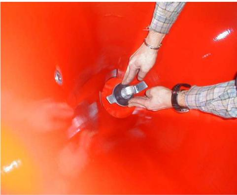
9) put the lower agitator and the holding rubber cap by checking it does not hit the hopper
