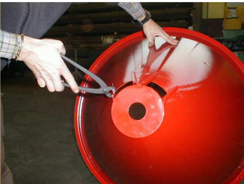
4) adjust the slides in case the gates do not close completely.
