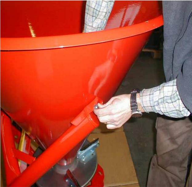
6) fix the frame to the hopper by 3 screws 10x25 and take care of putting all 3 screws so that the hopper hole is in a central position. After this tighten all the screws.
