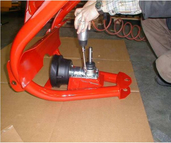
1) Tighten the gear box with 8X16 bolts
