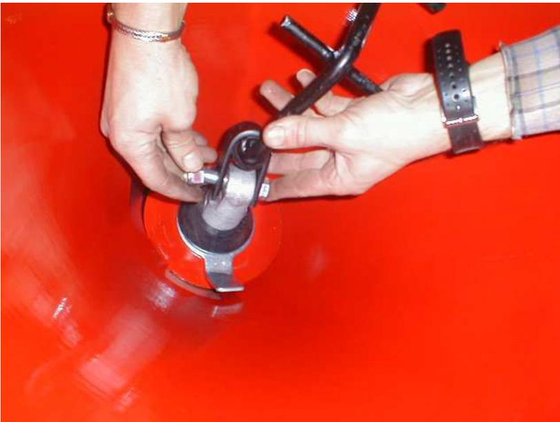
11) tighten the agitator at the entrainer bore.
