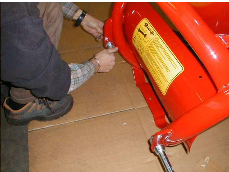
10 a) tighten the bolts-like-pins on the flanges
