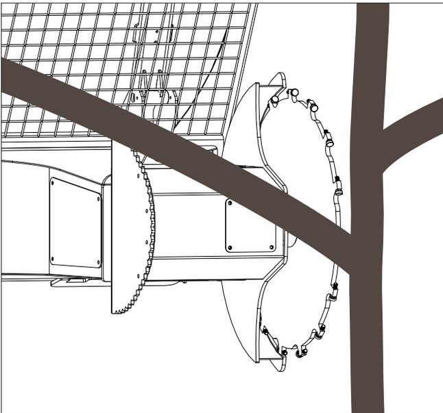
5. Operate hydraulics to move tree saw blade into brush, shrubs or tree.
