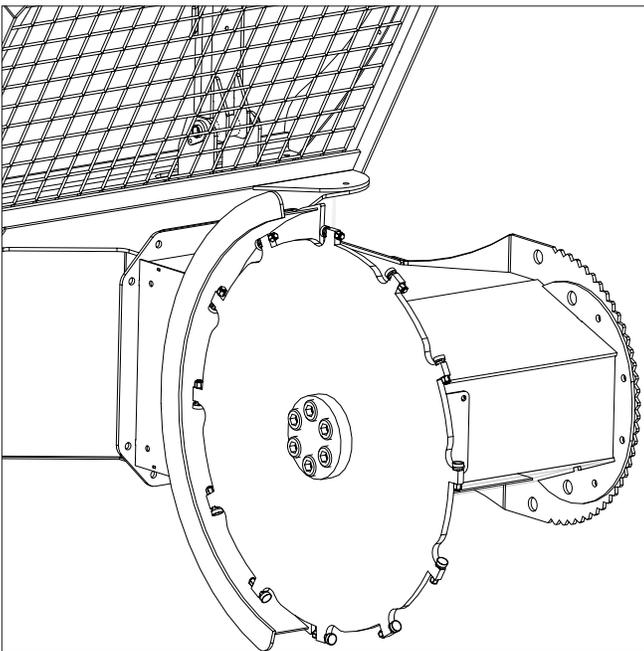
7. Install mounting hardware at eight locations (A) around cutting head and tighten securely.
