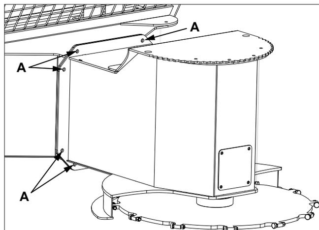
6. Support cutting head as needed and rotate 90 degrees clockwise or counter clockwise.
