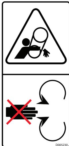
Decal D: D005039 ⚠️ WARNING - Pinch hazard. Keep back while machine is operating.
