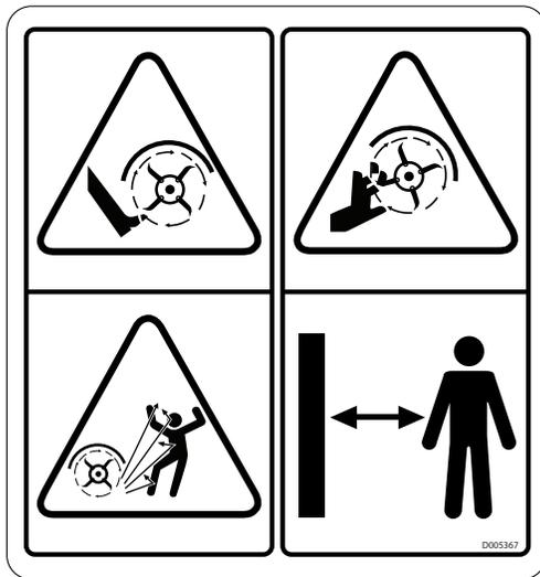
Decal C: D005230 ⚠️ WARNING - Rotating parts hazard. Do not reach into machine. Keep away from machine.
